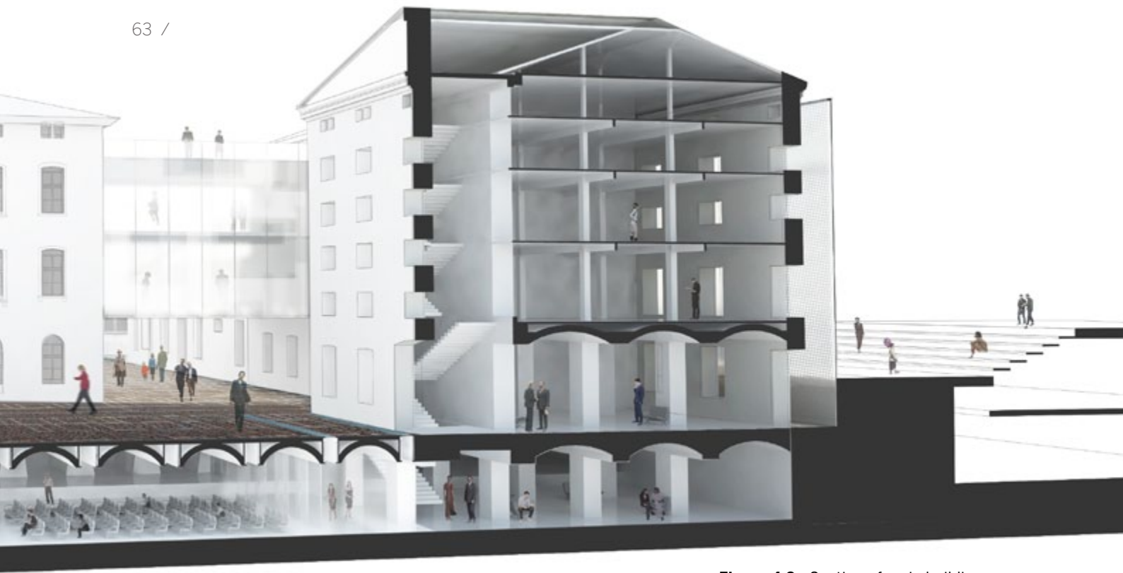
Figure 4.9 - Section of main building showing bridges and underground conference center
